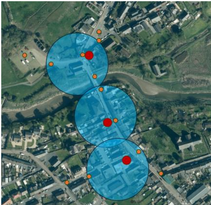
Figure 13 – Wi-Fi Hub Locations, Test Points and Ranges (Aerial Photo Source: OS Maps, 2024)
